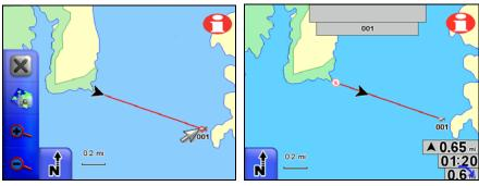
Navigating with the Go To Cursor command. At left, the boater has selected a waypoint (fish symbol) with the cursor and started navigating. The figure at right shows the straight-line navigation course after the cursor and toolbar have been cleared from the screen.
